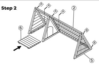
Position Back Panel (2) (no doorway) onto Left Panel, Middle Panel, and Right Panel and secure with 4- 2" screws (A) and 2- 11/2" screws (B). Place Floor Panel (6) onto Floor Support Bars between the Left and Middle Panels.
