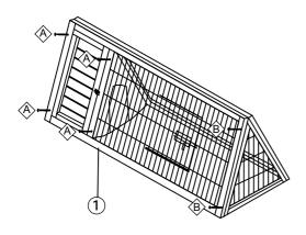
Position Front panel onto hutch and secure using 4-2" screws (A) and 2-11/2" screws (B).
