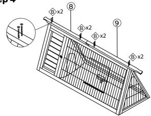
Secure the Ridge Cap Handle Left (8) and the Ridge Cap Handle Right (9) to the hutch assembly using 8-1½" screws (B).
