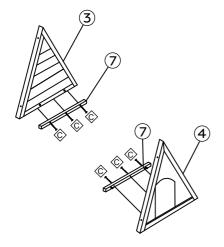
Install Floor Support Bars on Left Panel (3) and Middle Panel (4) using 6-11/4" Screws (C).
