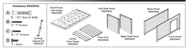
Step 1 Connect the Front Panel and the Back Panel to the Left and Right Side Panels using 8 - 23/4" nuts and bolts (A).
