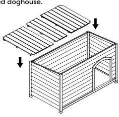
Tip: the corners of the two end pieces are notched to fit into the corners of the doghouse. The center piece does not have notches.
