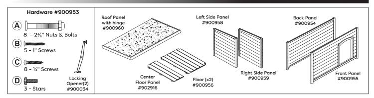
Connect the Front Panel and the Back Panel to the Left and Right Side Panels using 8 - 2<sup>3</sup>/<sub>4</sub>" nuts and bolts (A).
