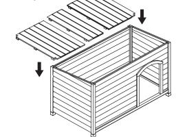
Tip: The corners of the two end pieces are notched to fit into the corners of the doghouse. The center piece does not have notches.
