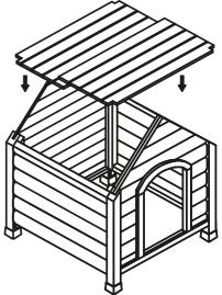
Step 4 Place the Roof Ridge Cap onto the Shingle Roof Panels and secure using 4 - 1" screws (C). Attach 3 - Star shaped bolts (D) onto the dog door frame in the threaded holes.
