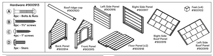
Step 1 Connect the Front Panel and the Back Panel to the Left Side Panel and Right Side Panel using 8 - Bolts & Nuts (A).
