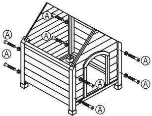
Step 3 Attach the Rigth Side Roof Panel and the Left Side Roof Panel to the assembled doghouse using 8 - 1%" screws (B).
