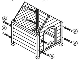
Attach the Rigth Side Roof Panel and the Left Side Roof Panel to the assembled doghouse using 8 - 1%" screws (B).
