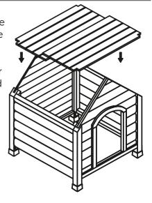
Place the Roof Ridge Cap onto the Shingle Roof Panels and secure using 4 - 1" screws (C). Attach 3 - Star shaped bolts (D) onto the dog door frame in the threaded holes.
