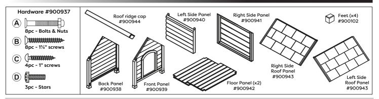
Connect the Front Panel and the Back Panel to the Left Side Panel and Right Side Panel using 8 - Bolts & Nuts (A).
