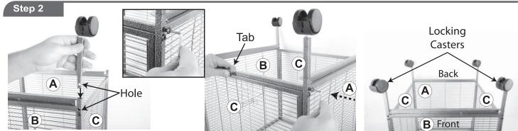
Insert the Casters into the Bottom Front (A) and Back (B) Wires, then connect both by screwing in bolts on each side(see inset image). Place the locking casters in the holes at the cage front. Flip the cage so the wheels are on the ground. Tip: the tabs on the support bars should be facing towards the outside.
