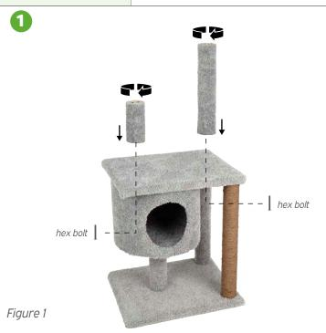
Using two Hex Bolts, attach the 16" Post and the 7" Post to the prebuilt base unit. (see figure 1)
