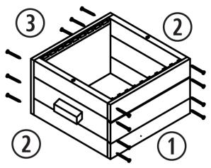
Assemble Hive Box Body by attaching a Hive Body Front and Hive Body Back onto two Hive Body Sides using  $14 - 1 \frac{1}{2}$ " (A) Screws.
